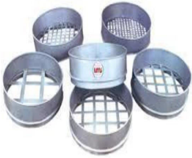
PLATE 4.4 A VIEW SET OF SIEVES FOR COARSE AGGREGATE
