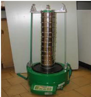
PLATE 4.3 A VIEW OF SET OF SIEVES FOR FINE AGGREGATE
