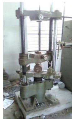
Fig 9: Split tensile strength testing at 5% Plastic at 14 days curing
