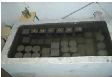
Fig 7: Curing of specimens for 7 days, 14 days and 28 days age
