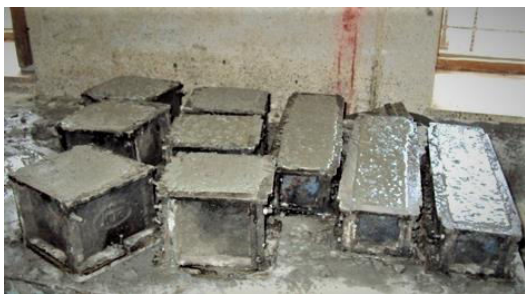
Fig 6: casting of samples (cubes and prisms)
