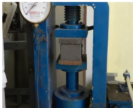
Fig 8: Testing of 10%MSW specimen at 7 days curing
