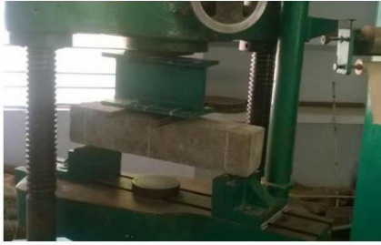
Fig 10: Flexural strength of prism specimen
