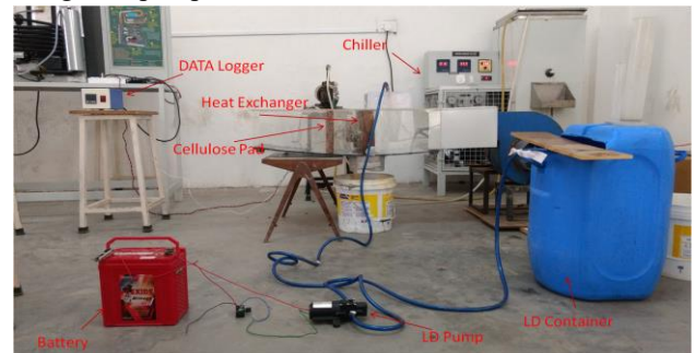
Fig. 2. Photograph of the experimental facility showing the VCR chiller, the data logger, the cellulose evaporative pad, the mini-channel heat exchanger on its stand, the LD container, the LD pump and the battery supply for the ancillary instrumentation.
