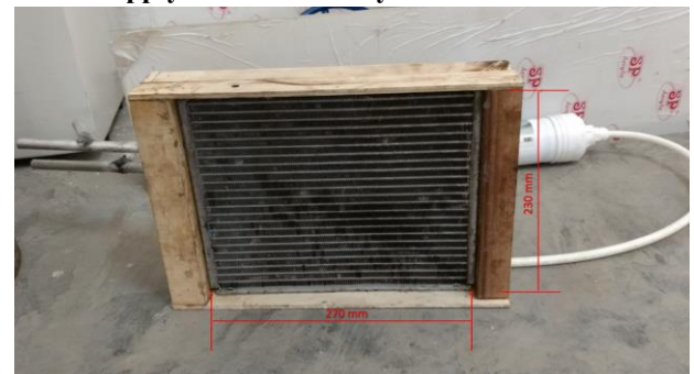
Fig. 3. Close-up view of the vertical finned-tube mini-channel coil used as the internally-cooled contacting device.
