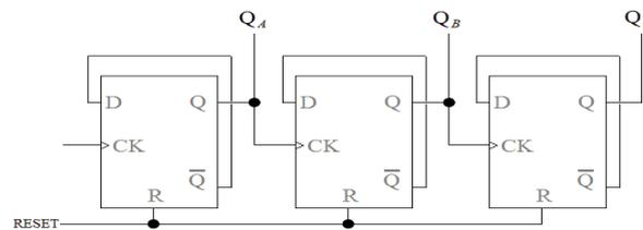
Fig. 5. . Asynchronous Down counter
