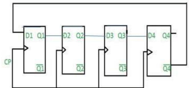
Fig. 3. . Johnson Counter based on TSPC D – flipflops.
