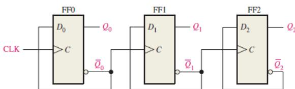
Fig. 4. Asynchronous UP counter
