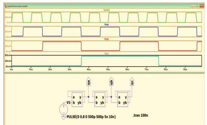
Fig. 12. Asynchronous UP Counter
