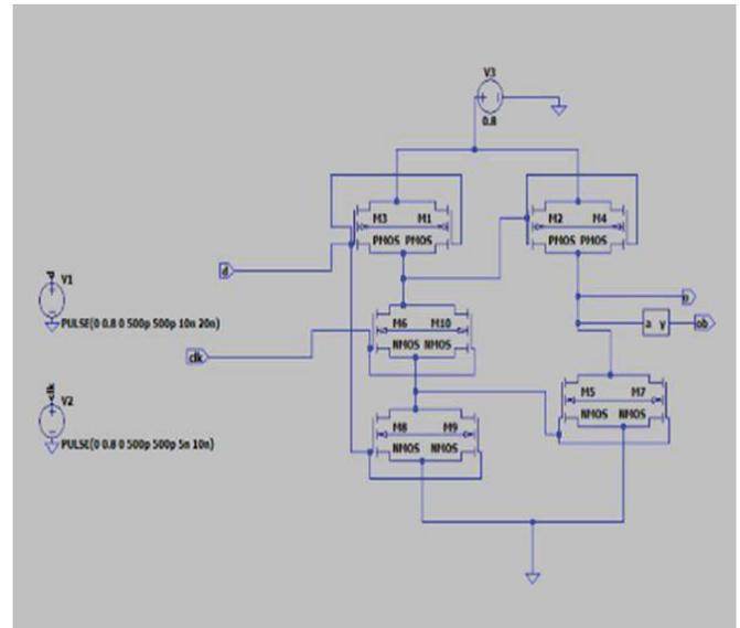
Fig. 2. TSPC based D – FlipFlop.
