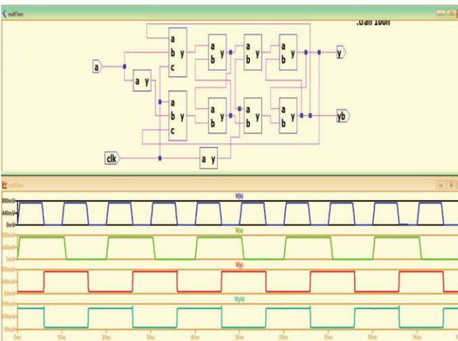
Fig. 7. D flip-flop (FinFET) Circuit and Output Waveforms.
