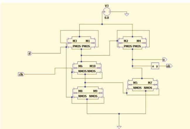
Fig. 8. TSPC D flip-flop (FinFET) Circuit
