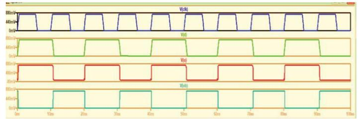
Fig. 9. TSPC D flip-flop (FinFET) output waveforms
