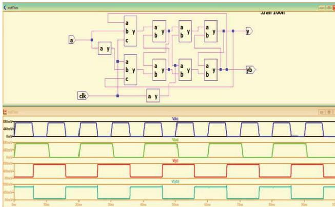
Fig. 6. D flip-flop (CMOS) Circuit and Output Waveforms.
