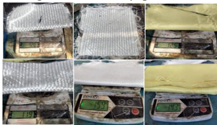
Figure 11 Various materials used for specimens (Kevlar, Carbon, E-glass, graphite powder, Hardner, Epoxy)
