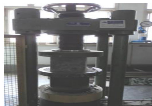
Figure.1 Experimental setup for compressive strength test
