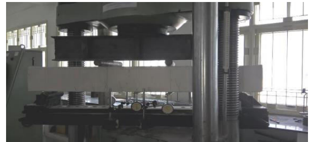
Figure.3 Experimental setup for flexural strength test
