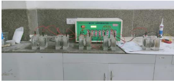
Figure.4 RCPT test conducting
