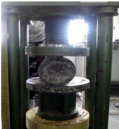
Figure.2 Experimental setup for split tensile strength test
