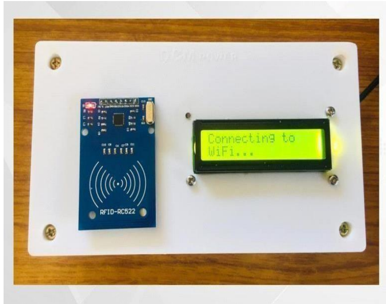
Fig.4.1. Module for scanning RFID tags and displaying response
