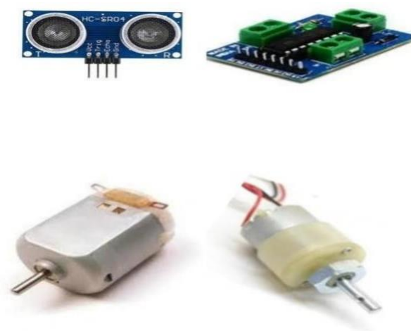
Figure 3: Sensor, L293D Motor drive, Dc motor and Gear Motor
