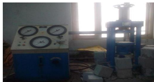
Figure: 3.3 Compressive testing machine
