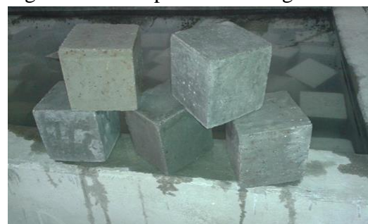
Figure: 3.4 Concrete cube specimens
