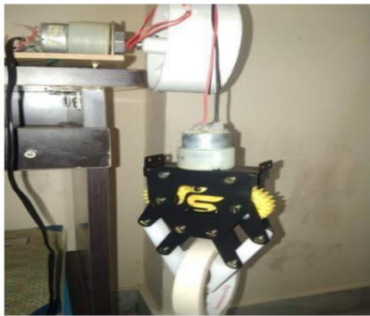
FIG 6 OBJECT PICK UP WITH HELP OF GRIPPER
