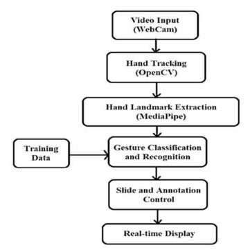
Fig 1: Architecture Diagram.
