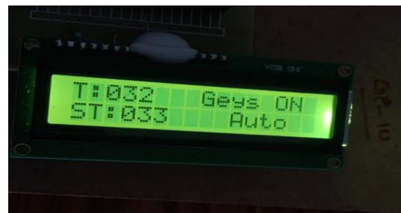
Figure 6. Automatic Mode of Operation- Geyser ON
