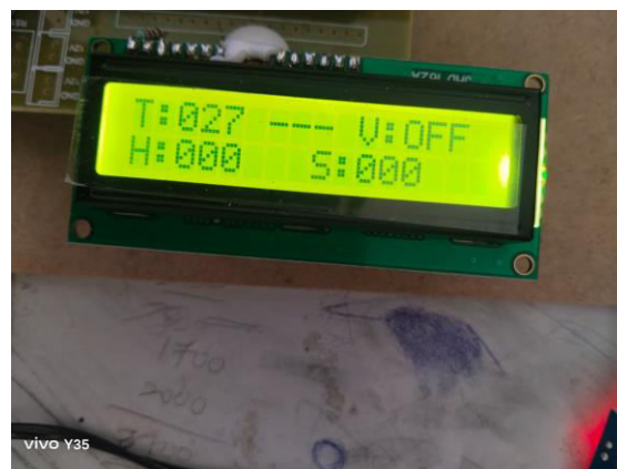
Figure 6. LCD Display Showing Real-Time Sensor Parameters
